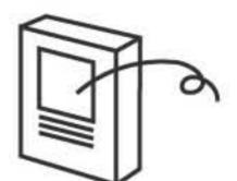
Protected against sprays of water up to 60 degrees from the vertical. Limited ingress permitted for three minutes.
