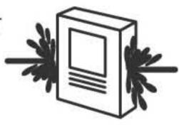
SIRONGARA Protection against the effects of immersion in water between 15cm and 1m for 30 minutes.
